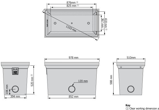
Key (1) Clear working dimension at pit base (2) Clear working dimension at pit opening (3) Clear working dimension beneath rebate
