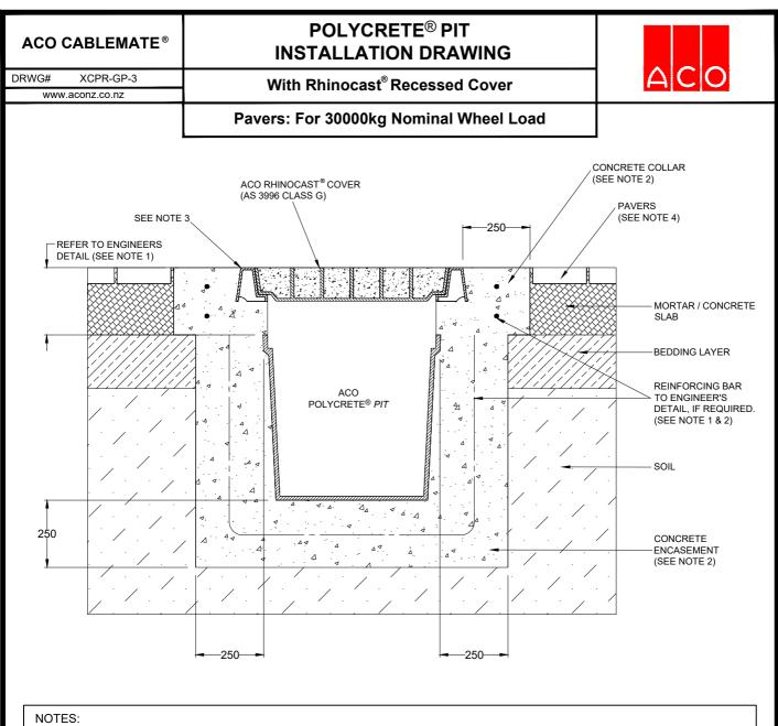
1. Specific site conditions may require an increase in these dimensions or reinforcement. It is the customer's responsibility to ensure the installation drawing is detailed for the application and the pit structure is protected from undue stress. *Engineering advice may be required.*
